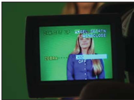
DVD. Fig. 6 -illustrates the subject in the Camcorders viewfinder against a screen and the dialogue explains how to light and use the Zebra function on the Camcorder to make sure the lighting of the screen is correct.
